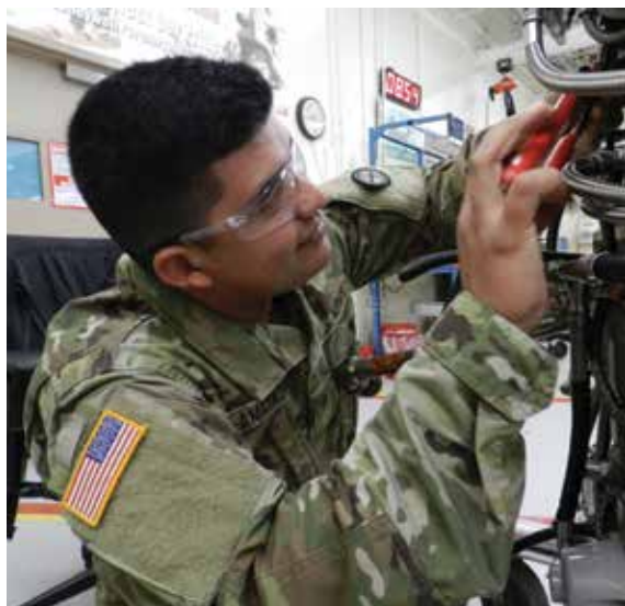
PFC Randall Amayadias, of the Utah National Guard, puts a locking tab on a T55 at Corpus Christi Army Depot’s engine shop where he practices maintaining CH-47 engines.
