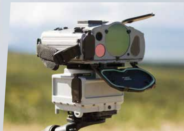
The Joint Effects Targeting System (JETS), at less than 5.5 pounds, weighs less than half of the Lightweight Laser Designator Rangefinder and offers greater precision than the Vector 21 Laser Target Locator.
