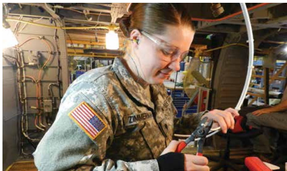
SPC Ashtyn Zimmerman of the D Company, 2-211th General Support Aviation Battalion trims wire from a D-Ice Box to prevent frost on UH-60 rotor blades during avionics training at Corpus Christi Army Depot.
