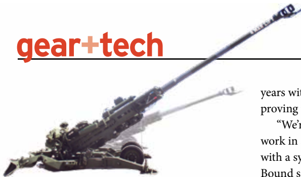
The modified 155 mm M777A2 Howitzer, front, will have a range more than double that of the current version, which can be seen in the background of the Extended Range M777A2.
