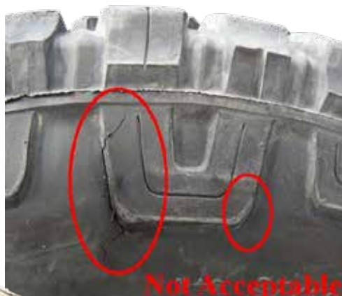
Examples of defects found in HMMWV tires during safety inspection of vehicles in Kentucky.
